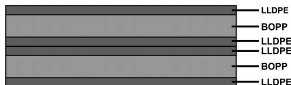
Figure 12. Schematic showing the composition of Strand 78.
