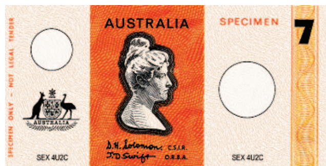
Figure 10. Experimental $7 note printed on Strand 75 with two circles cut for OVDs.
